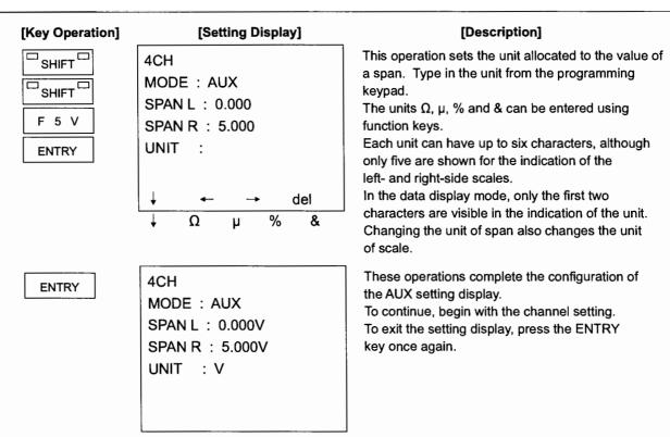
**Note:** After having finished with the AUX setting display using the procedure noted above, follow the readout (READ) procedure in Subsection 6.4.13, "IC Memory Card Setting," to read measurement data.
